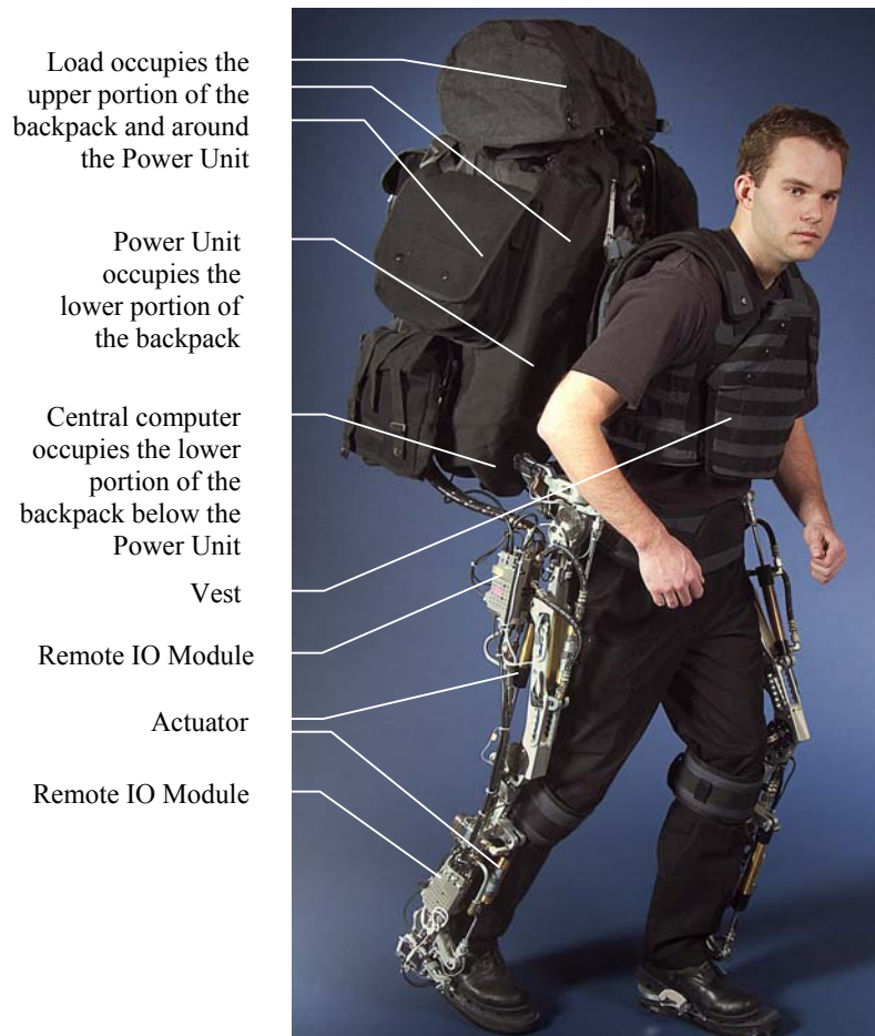
The first prototype of Berkeley Lower Extremity Exoskeleton (BLEEX)
