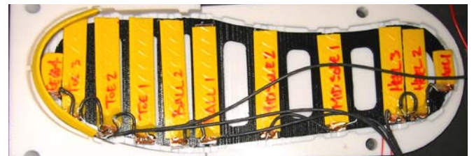
Fig. 15: Original Foot Switches Designed with Digital Tape Switches. Note the four "zones": toe, ball, midsole, and heel.
