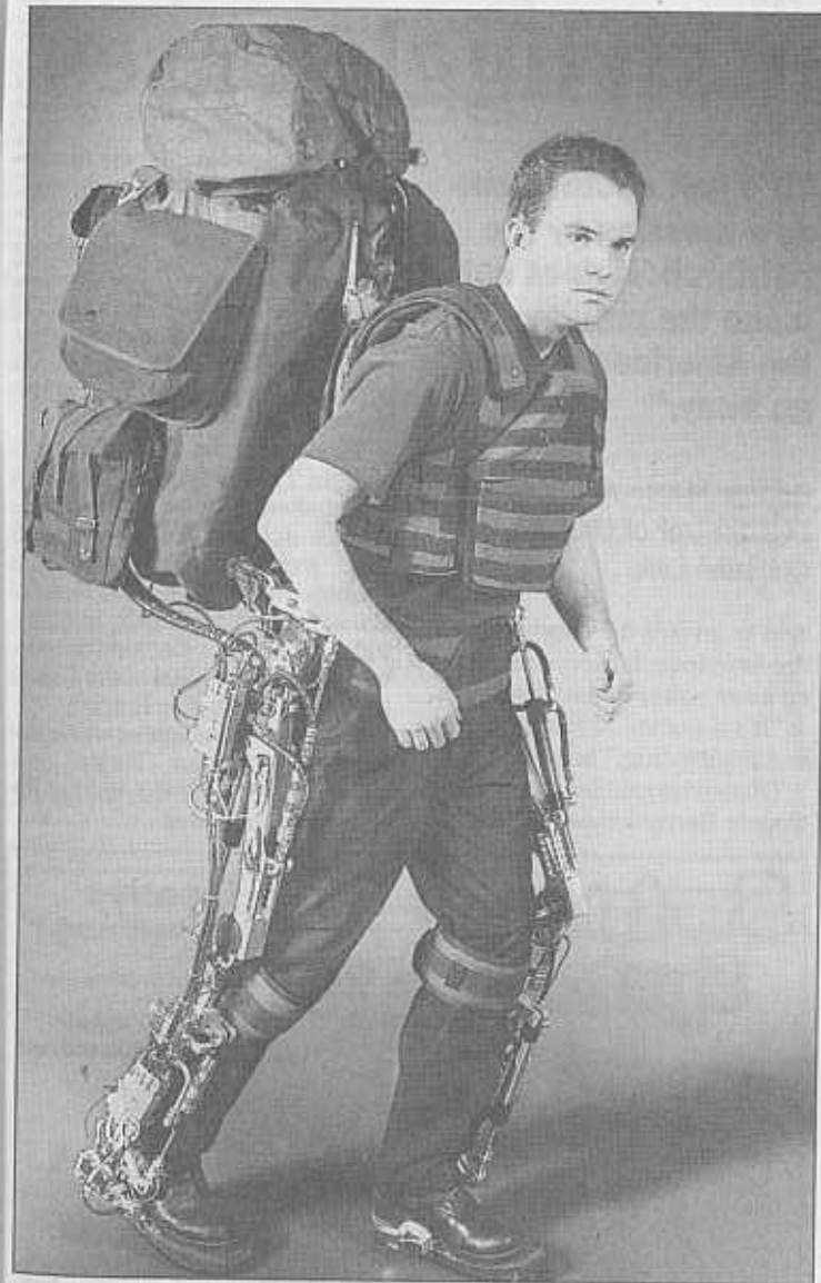
The Associated Press from the University of California Berkeley The BLEEX consists of a pair of robotic leg braces attached to a pair of boots with a power unit and backpack.
