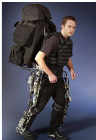
A model is seen wearing the BLEEX, (Berkeley Lower Extremity Exoskeleton), which is ultimately intended to assist people such as soldiers or firefighters bearing heavy loads for long distances.
