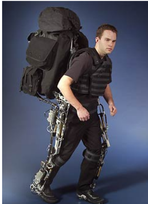
The Berkeley Lower Extremity Exoskeleton (BLEEX) helps lighten the load for the human user. (UC Berkeley photo)
