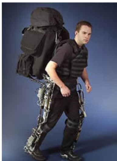
The Berkeley Lower Extremity Exoskeleton can be used to carry an extra 32 kilograms (Image: US Berkeley)
