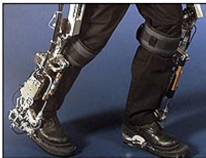
The exoskeleton allows people to carry heavy loads
