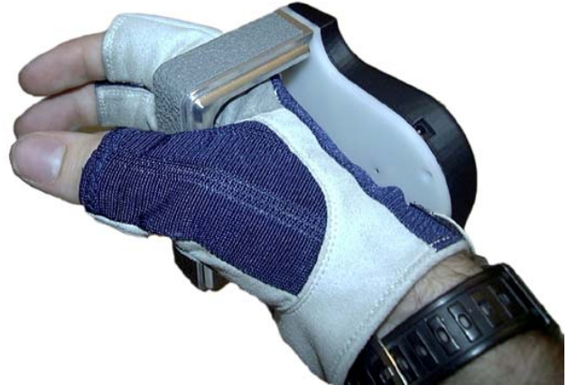
Fig. 1: A prototype instrumented glove is designed to measure the wearer contact force with a robot and broadcast a set of control signals representing the contact force for moving the robot.
