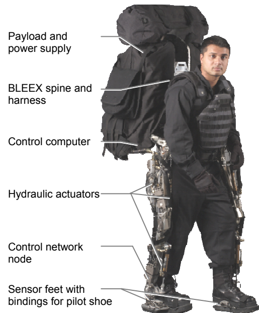
Fig. 1: Berkeley Lower Extremity Exoskeleton (BLEEX) and pilot. exoskeleton (commonly referred to as BLEEX) is comprised of two powered anthropomorphic legs, a power unit, and a backpack-like frame on which a variety of heavy loads can be mounted. This system provides its pilot (i.e. the wearer) with the ability to carry significant loads on his/her back with minimal effort over any type of terrain. BLEEX allows the pilot to comfortably squat, bend, swing from side to side, twist, and walk on ascending and descending slopes, while also offering the ability to step over and under obstructions while carrying equipment and supplies. The overall concept of this lower extremity exoskeleton is that the human provides an intelligent control system for the exoskeleton while the exoskeleton actuators provide most of the strength necessary for walking [1,2].
