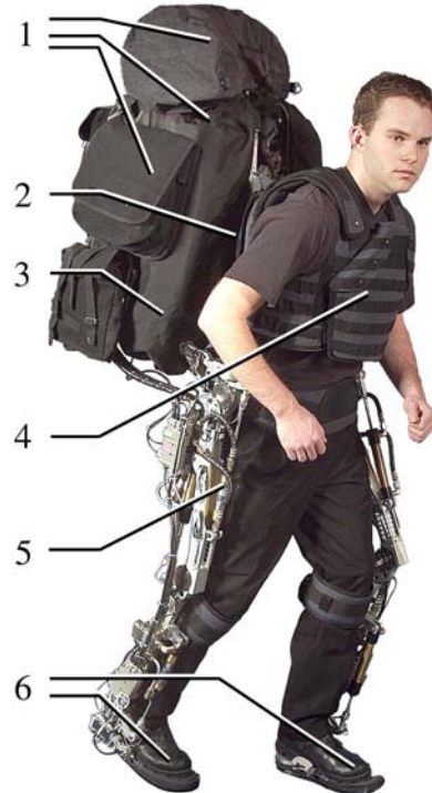
Fig. 1 Berkeley Lower Extremity Exoskeleton (BLEEX) and pilot Ryan Steger. 1: Load occupies the upper portion of the backpack and around the Power Unit; 2: Rigid connection of the BLEEX spine to the pilot's vest; 3: Power unit and central computer occupies the lower portion of the backpack; 4: Semi-rigid vest connecting BLEEX to the pilot; 5: One of the hydraulic actuators; 6: Rigid connection of the BLEEX feet to the pilot's boots. More photographs can be found at http://bleex.me.berkeley.edu
