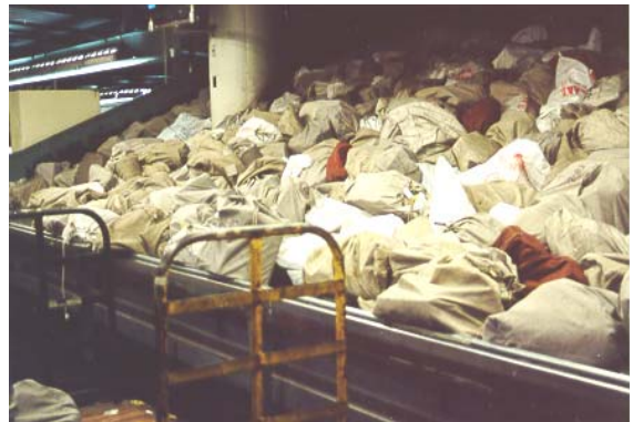
Figure 1: An example of a USPS Distribution Center in Northern California where thousands of sacks are unloaded off a large slide and either emptied directly onto conveyor belts, or loaded onto carts by hand
